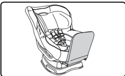
3. Recline the unoccupied child seat to position 3 and place rear-facing on the vehicle seat (see page 24). Ensure that no more than 7.5 cm (3 in.) of the base hangs over the edge of the vehicle seat.
