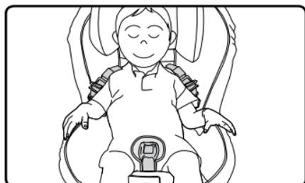
**IMPORTANT:** Adjust the harness to fit the clothes the child is wearing. Remove bulky coats, jackets and/or bulky sports equipment before putting the child in the child seat.
