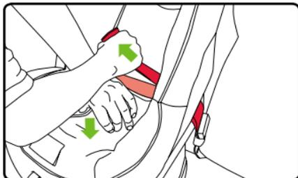
9. Attach the tether to a designated anchor (see vehicle owner's manual) and remove all slack (see page 29). Wrap excess webbing in the elastic strap and store in tether storage pouch.
