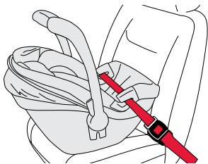
Carrier Only Installation with Lap Belt
