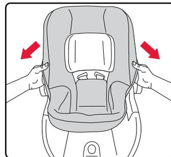
2. Pull the harness adjuster strap through cover and fit the cover around harness adjust button.
